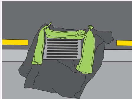
Stormwater protection on level ground
