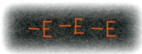
A single orange line shows an individual cable, and you must hand dig within 300mm each side.
