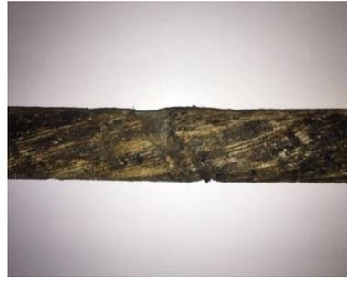
**Figure 4 – Examples of 11 kV cables at Centerport that pulled apart and then came back together.**
