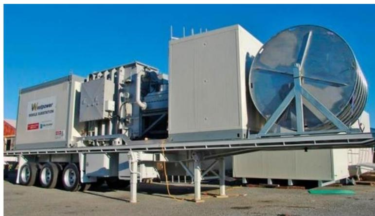
Figure 8 – Mobile Substation
