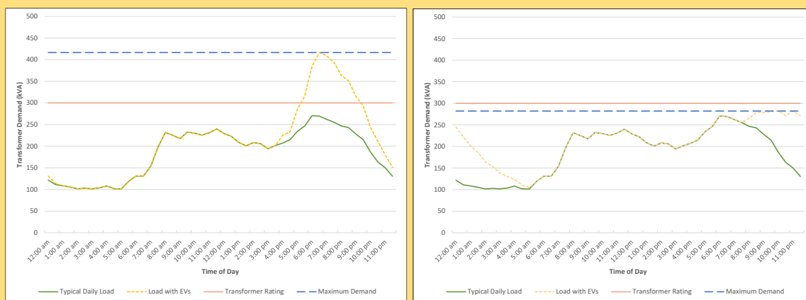
Figure 4-7 Example Impact of Large EV Charger Management on LV Network Capacity Without Charger Coordination (Left) and With Charger Coordination (Right)
