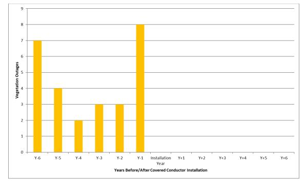
Figure 7-8 Aggregated Vegetation Outages in Covered Conductor Areas
