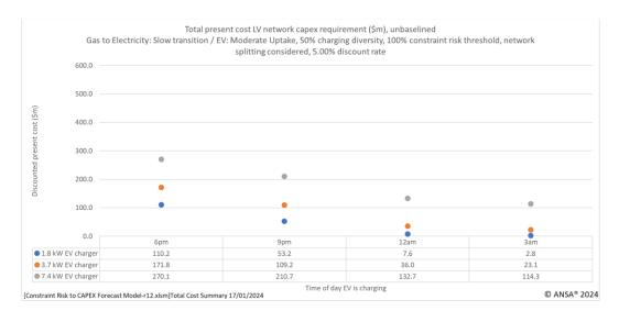
Figure 9-39 Impact of Charging Behaviour on LV Reinforcement CAPEX
