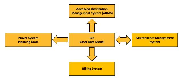
Figure 11-2 GIS Centrality to Asset Data Model
