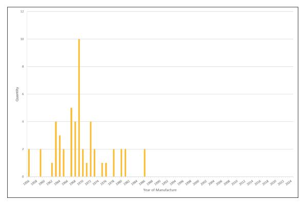
Figure 8-7 Age Profile of Zone Substation Transformers
