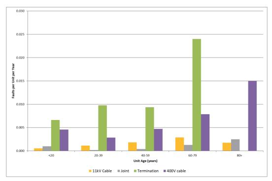
Figure 8-20 Cable Failure Rate by Age
