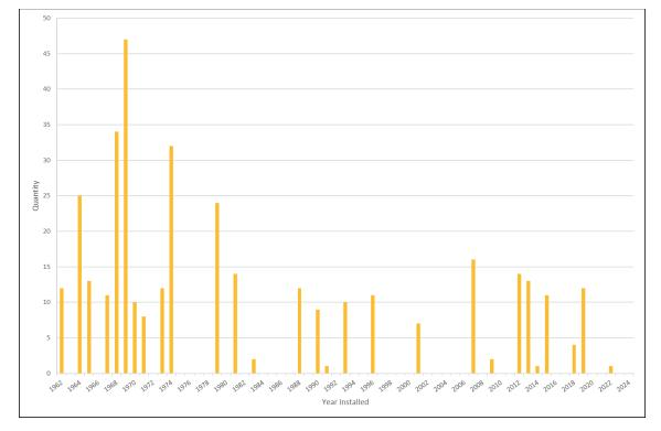
Figure 8-9 Age Profile for Zone Substation Circuit Breakers
