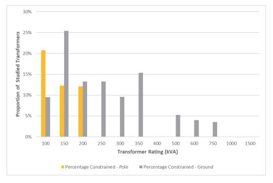
Figure 9-43 Constrained Transformers by Rating as Proportion of Fleet
