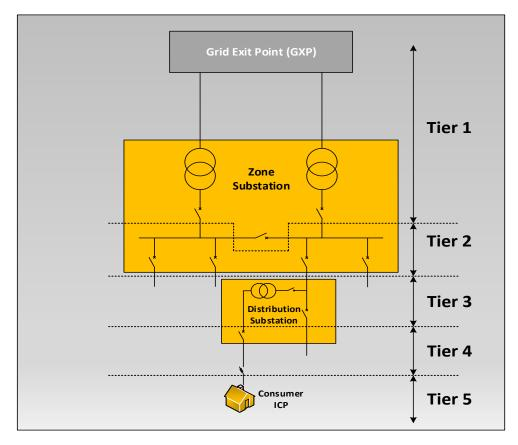
Figure 8-32 WELL Protection Tier System
