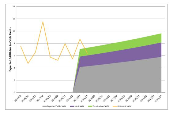
Figure 8-21 Forecast 11kV Cable Fleet Performance Trend without Intervention
