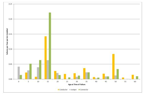
Figure 8-17 Overhead Conductor and Connector Failure Rate by Age
