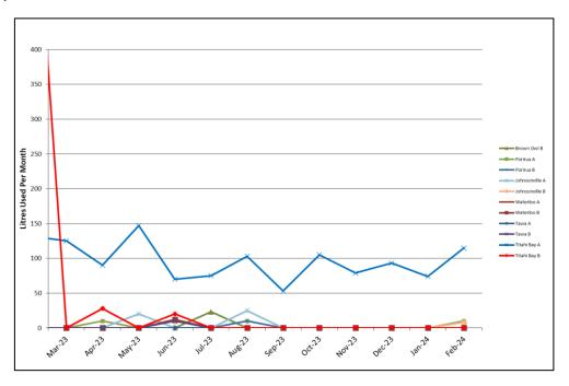
Figure 8-5 Monthly Fluid-Filled Cable Leakage
