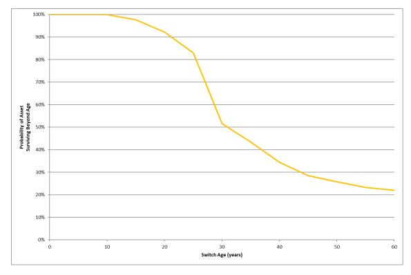
Figure 8-31 Overhead Switch Survival Curve
