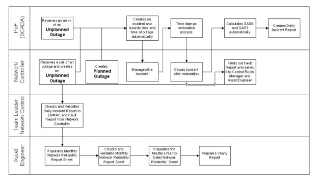
Figure 6-7 WELL Reliability Measurement Process
