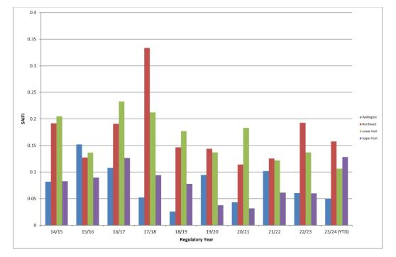
Figure 6-13 Unplanned SAIFI Performance by Network Area
