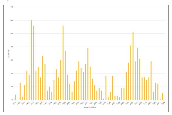
Figure 8-25 Age Profile for Distribution Circuit Breakers
