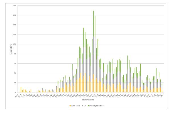
Figure 8-18 Age Profile of Distribution Cables
