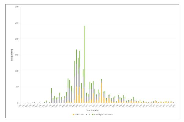
Figure 8-14 Age Profile of Distribution Overhead Line Conductors
