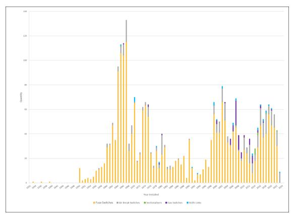
Figure 8-30 Age Profile of Overhead Switchgear and Devices
