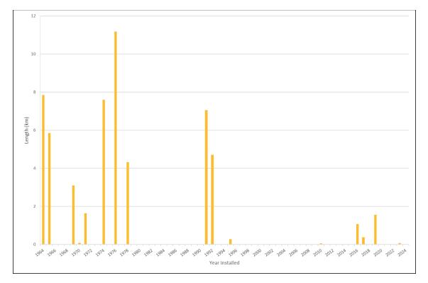
Figure 8-13 Age Profile of Subtransmission Line Conductors
