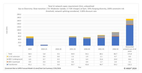
Figure 9-44 Forecast LV Reinforcement CAPEX to 2050
