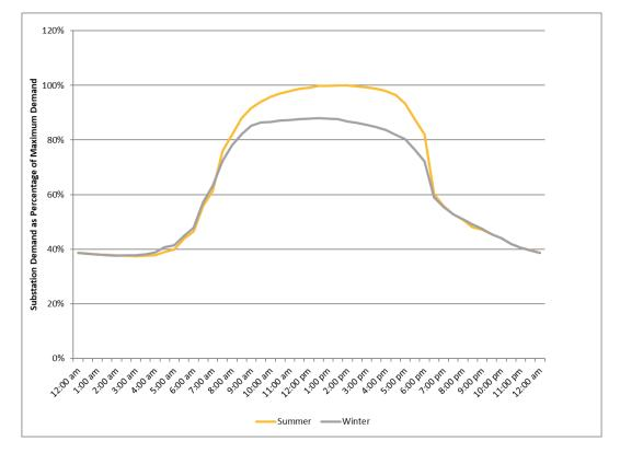
Figure 9-5 Typical CBD Zone Substation Daily Load Profile
