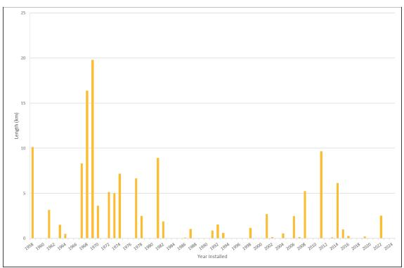
Figure 8-3 Age Profile of Subtransmission Cables
