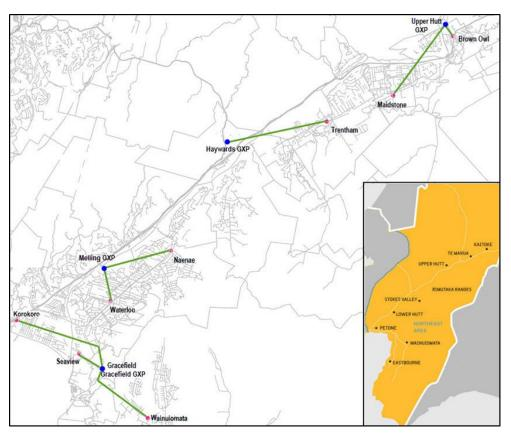
Figure 3-6 Wellington Northeastern Area Subtransmission Network
