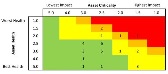
Figure 8-10 Zone Substation Switchboard Health-Criticality Matrix
