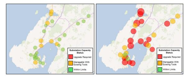
Figure 4-14 Change in Zone Substation Demand vs Capacity from 2023 (Left) to 2033 (Right)
