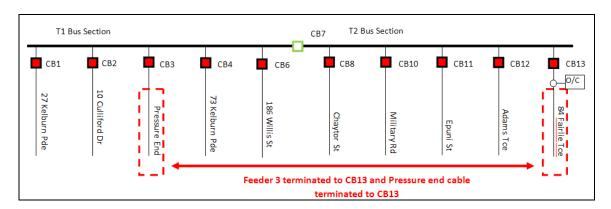
Figure 5-53 Re-configuration of the University zone substation
