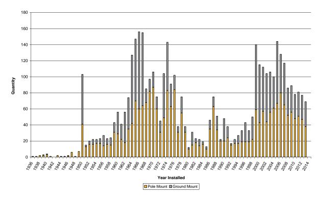
Figure 3-39 Age Profile of Distribution Transformers
