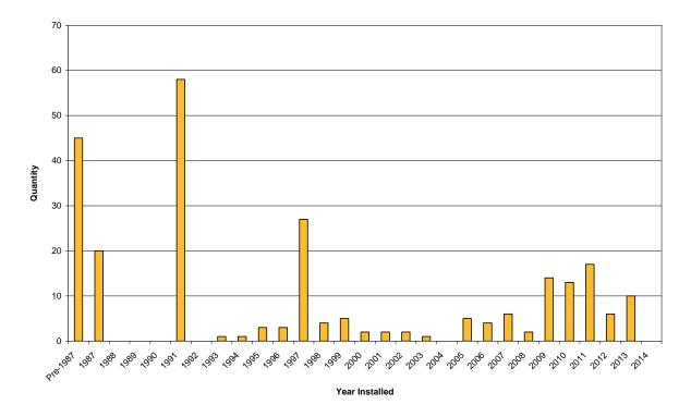
Figure 3-28 Age Profile of SCADA RTUs
