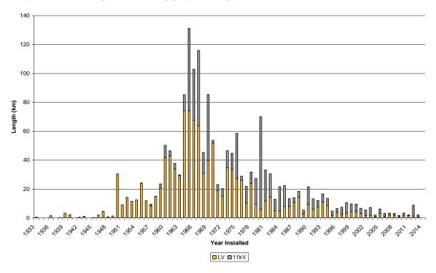
Figure 3-33 Age Profile of Distribution Overhead Line Conductors
