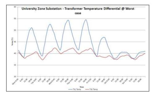
Figure 5-52 University zone substation T1 and T2 temperature differential
