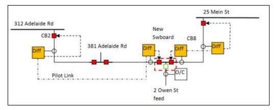
Figure 5-45 Proposed re-configuration of 25 Mein St substation
