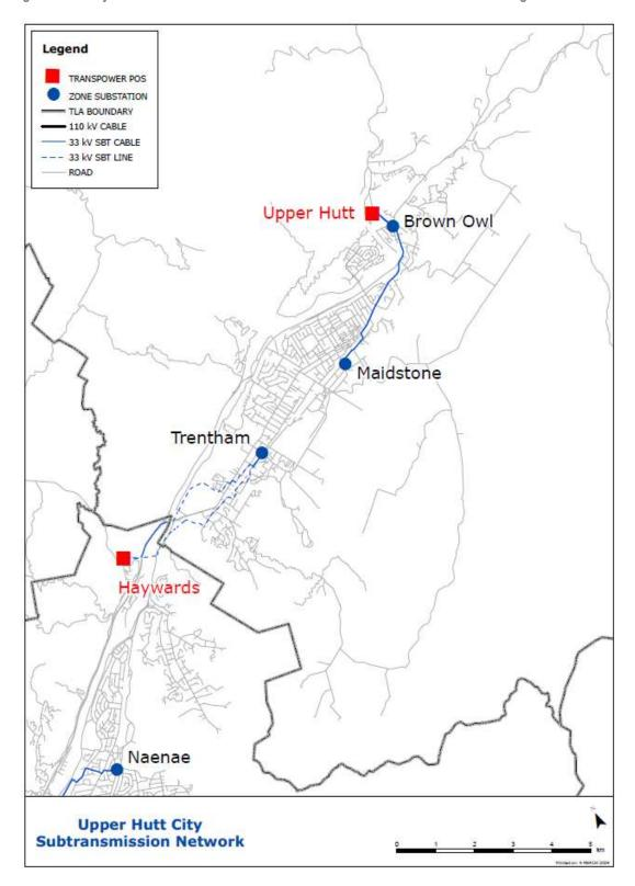
Figure 3-10 Upper Hutt City Subtransmission Network
