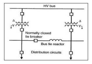
Figure 5-35 Typical Bus Tie Reactor Arrangement
