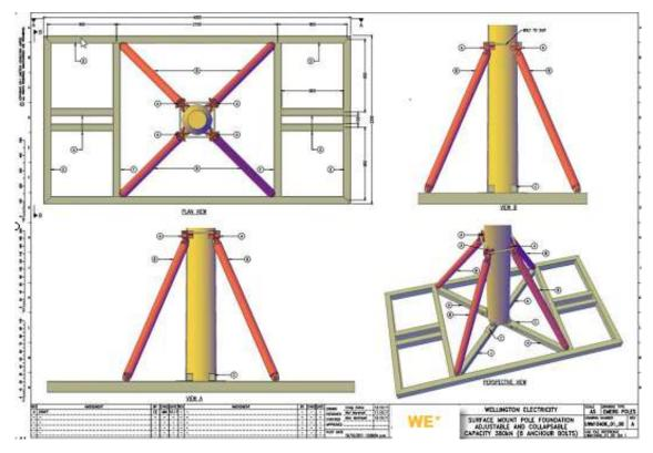
Figure 8-20 33kV Pole Structure Supports (Example only)
