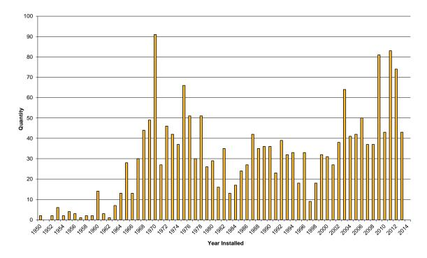
Figure 3-41 Age Profile of Ground Mounted Distribution Switchgear
