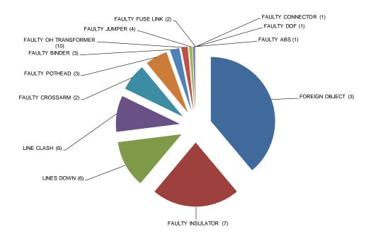
Figure 7-6 SAIDI impact of the Overhead equipment failure – Fault cause
