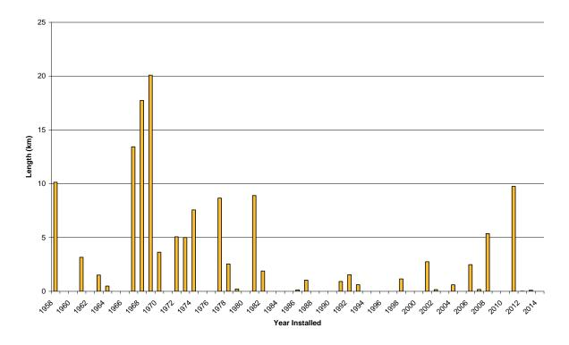
Figure 3-16 Age Profile of Subtransmission Cables
