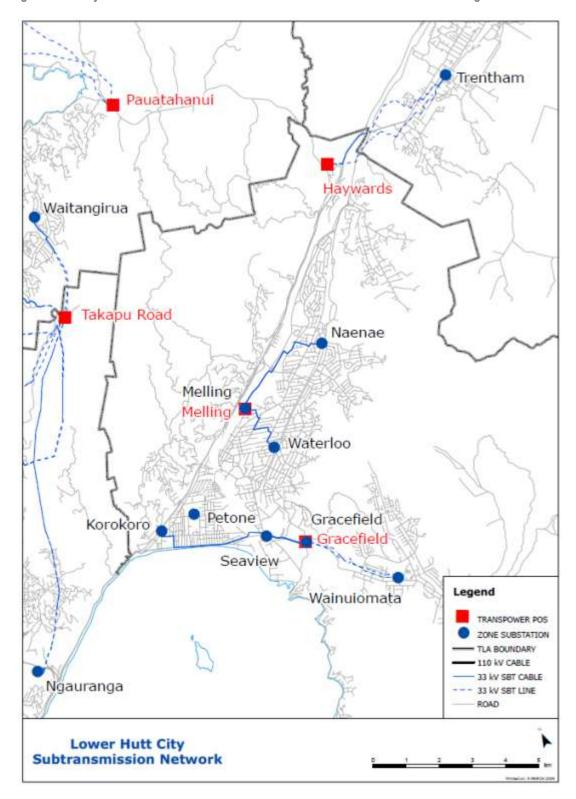
Figure 3-8 Lower Hutt Subtransmission Network
