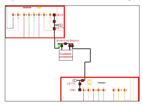
Figure 5-29 Proposed ring feed to Customer data centre facility
