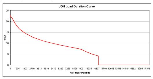
Figure 8-7 Load Duration Curve for Johnsonville Zone Substation
