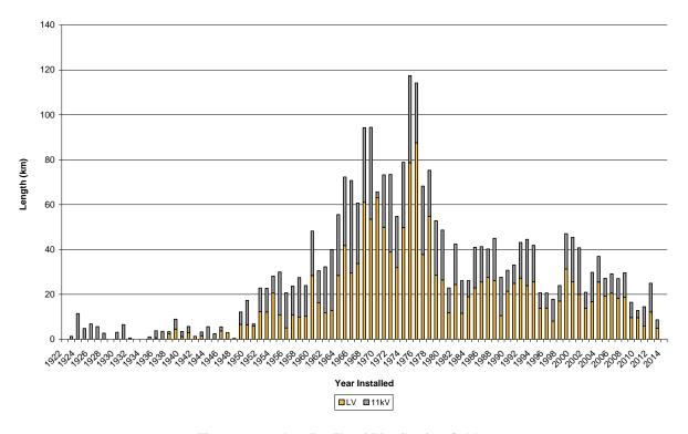
Figure 3-44 Age Profile of Distribution Cables
