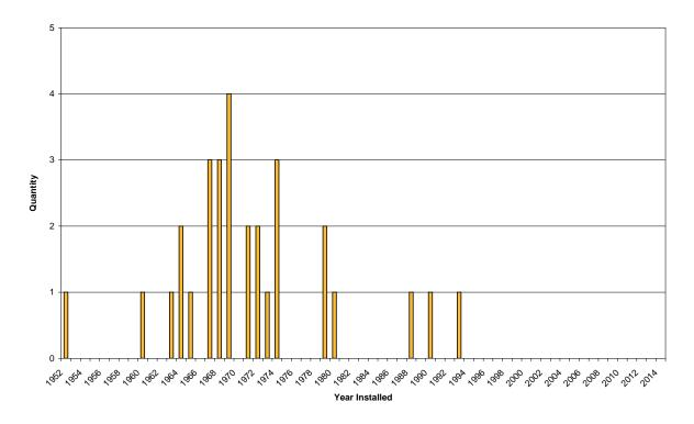
Figure 3-20 Age Profile of Zone Substation Buildings
