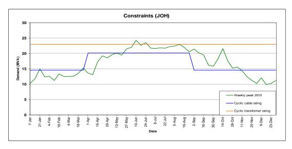
Figure 8-5 Johnsonville subtrans N-1 Equipment and Zone Tx Capacity Constraints (2010)
