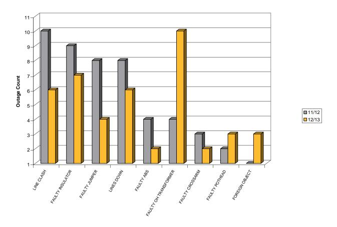
Figure 7-7 Outage Count of Overhead equipment failure – Fault cause
