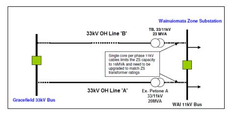
Figure 5-32 Wainuiomata Zone Substation Layout
