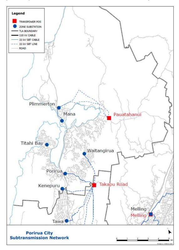
Figure 3-9 Porirua City Subtransmission Network
