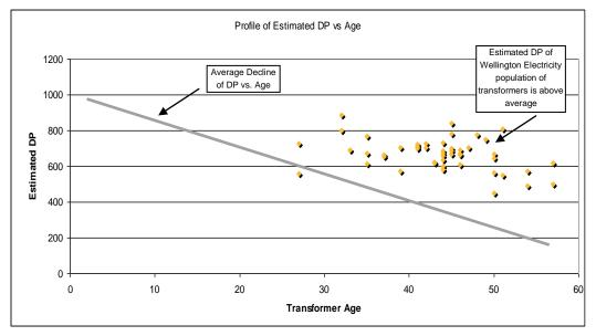
Figure 6-12 Profile of Estimated DP vs. Age (Based on 2009 Testing)
