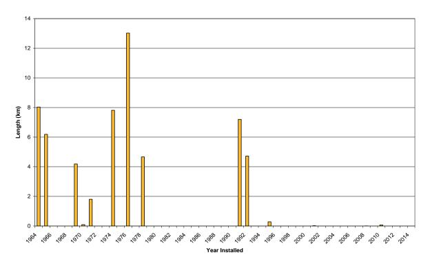
Figure 3-19 Age Profile of Subtransmission Lines
