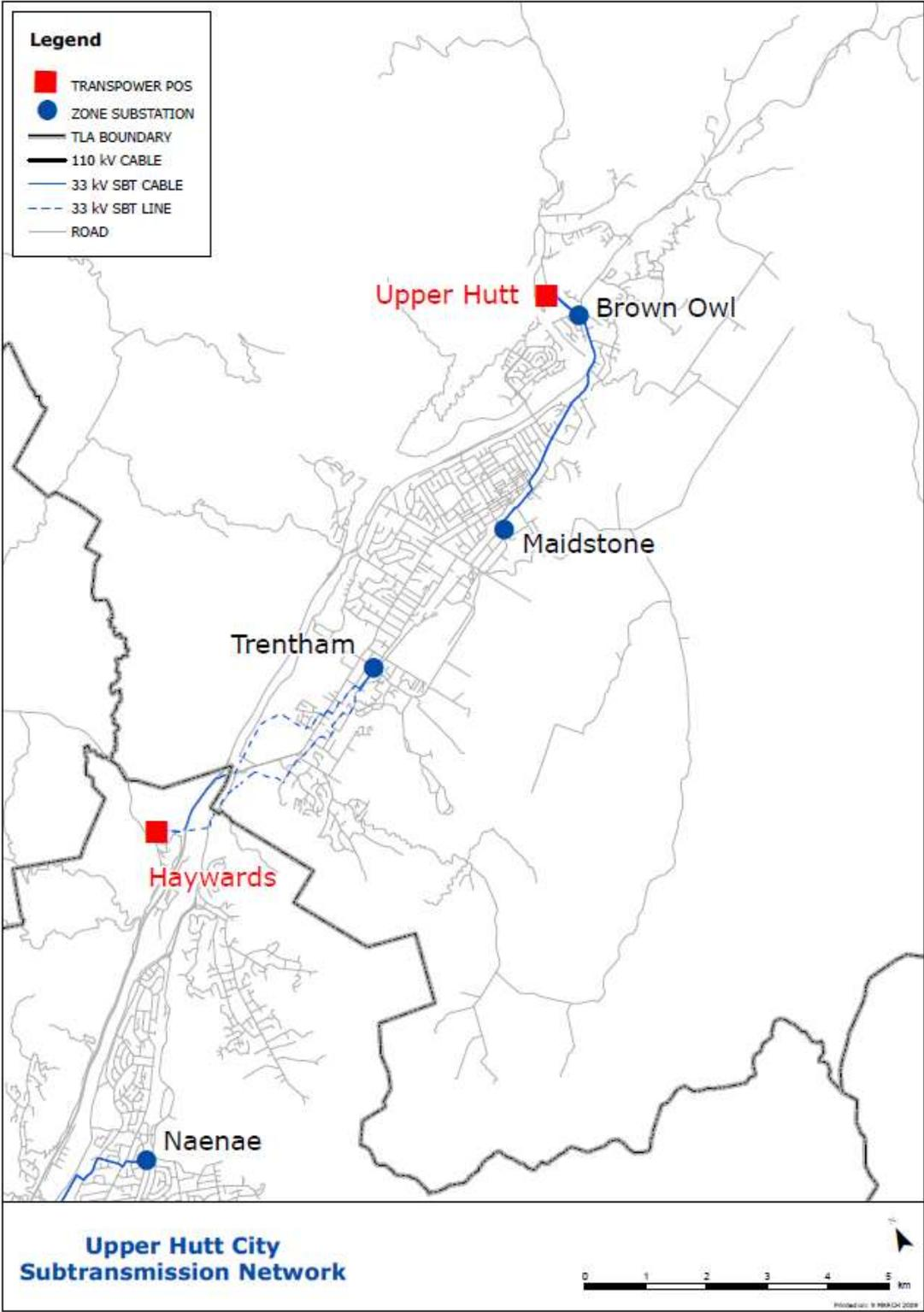
Figure 3-10 Upper Hutt City Subtransmission Network
