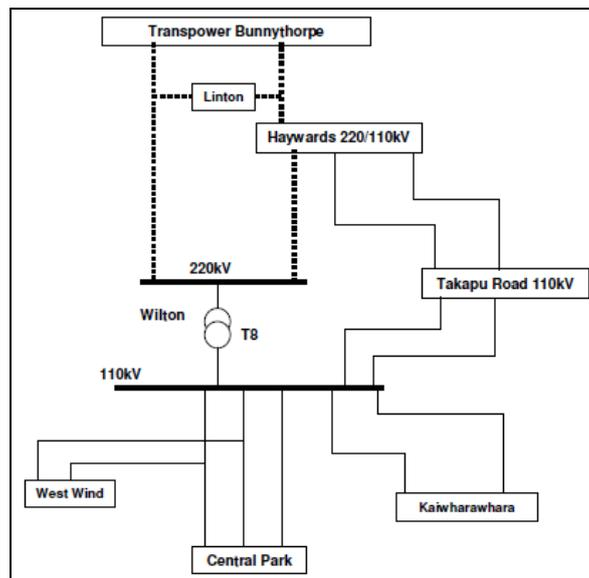
Figure 5-15 Transpower 220 & 110kV Network supplying Wellington Network layout
