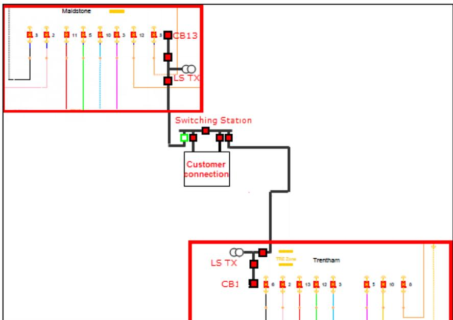
Figure 5-29 Proposed ring feed to Customer data centre facility
