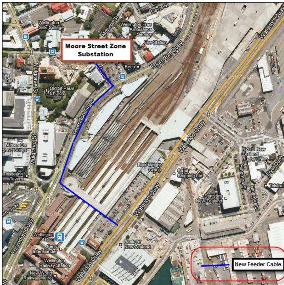
Figure 5-49 New feeder layout from Moore Street to Waterloo Quay
