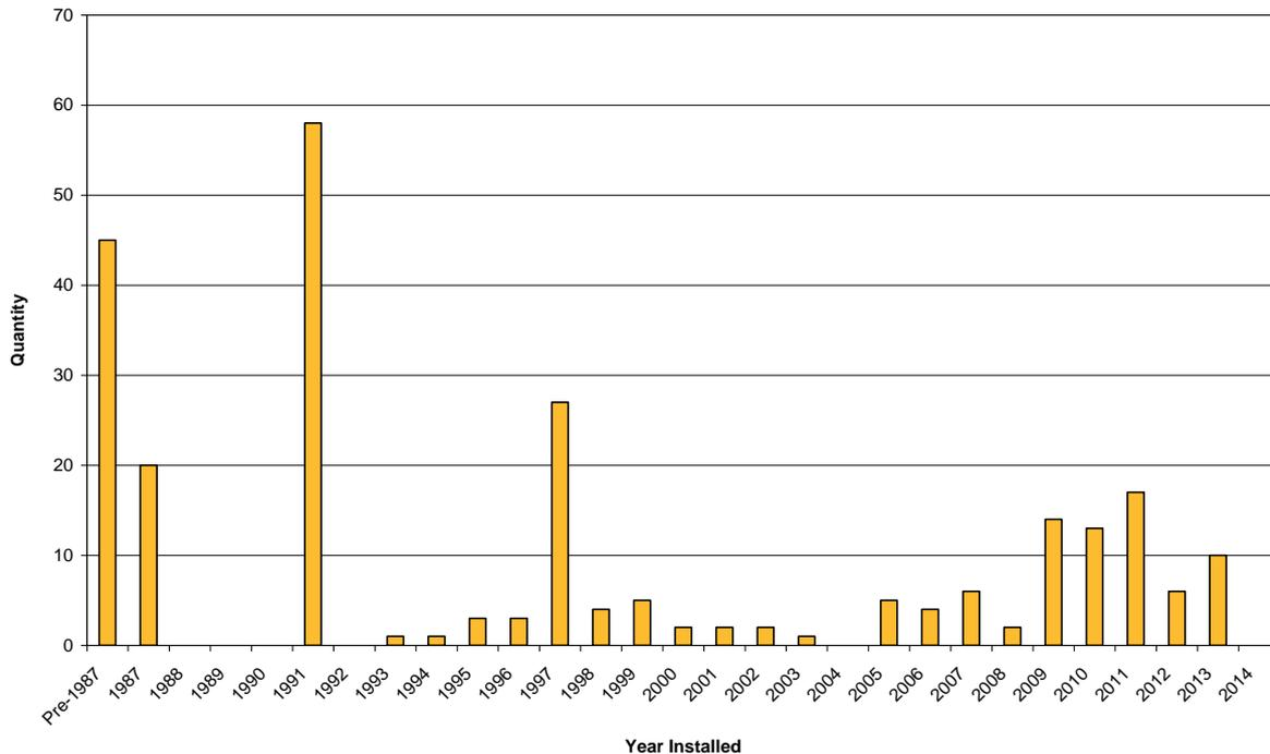
Figure 3-28 Age Profile of SCADA RTUs
