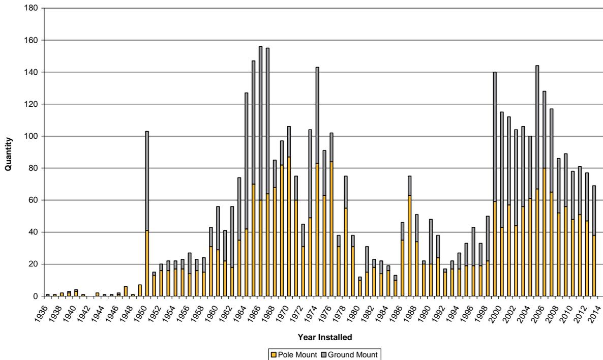
Figure 3-39 Age Profile of Distribution Transformers
