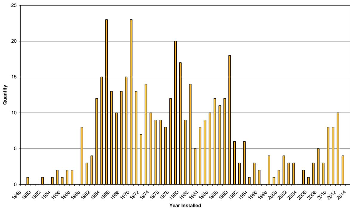
Figure 3-24 Age Profile for Switchboards
