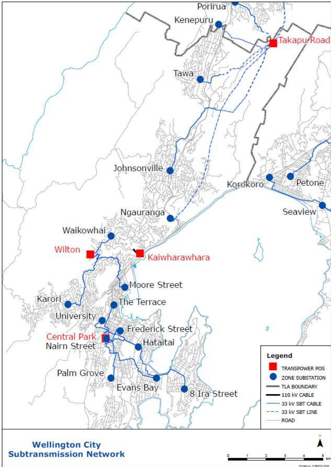
Figure 3-11 Wellington City Subtransmission Network
