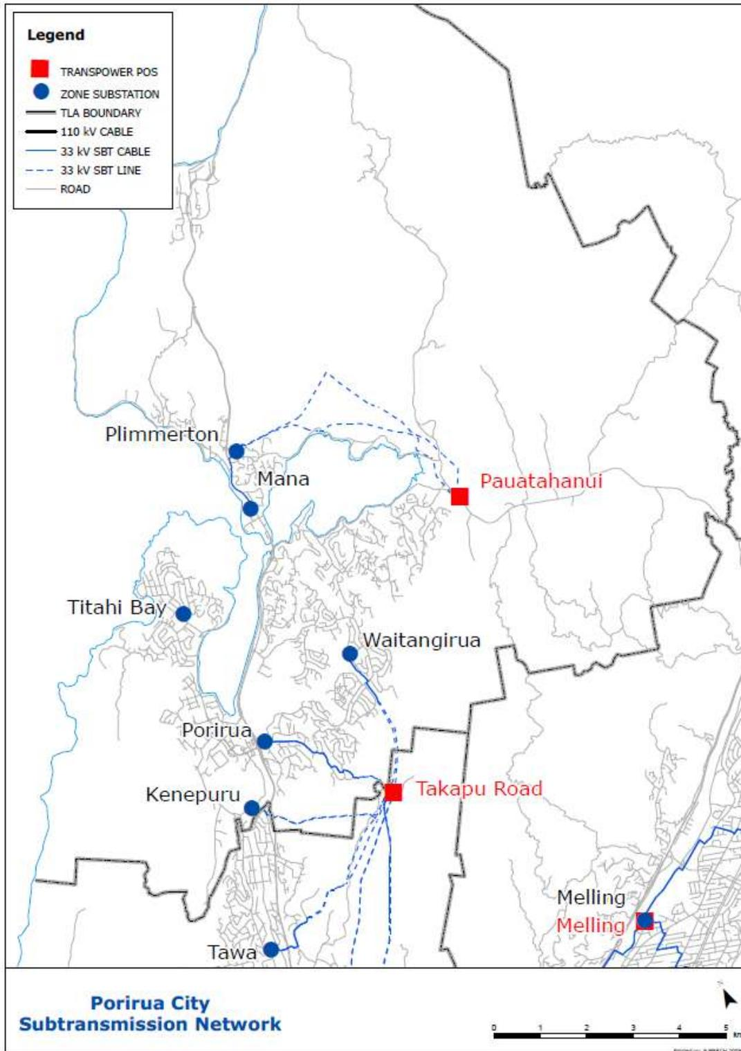
Figure 3-9 Porirua City Subtransmission Network
