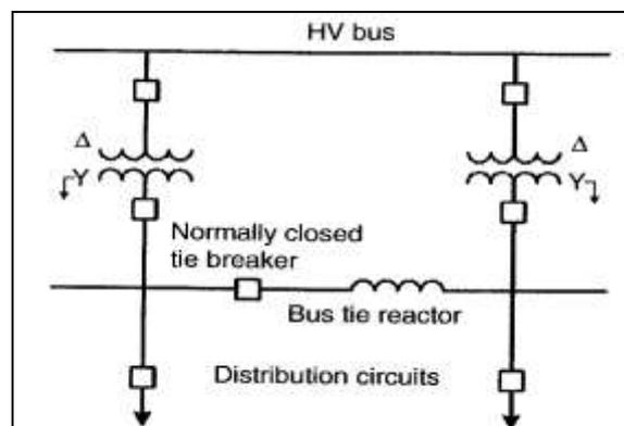
Figure 5-35 Typical Bus Tie Reactor Arrangement
