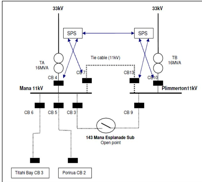
Figure 5-21 Special protection scheme logic at Mana and Plimmerton
