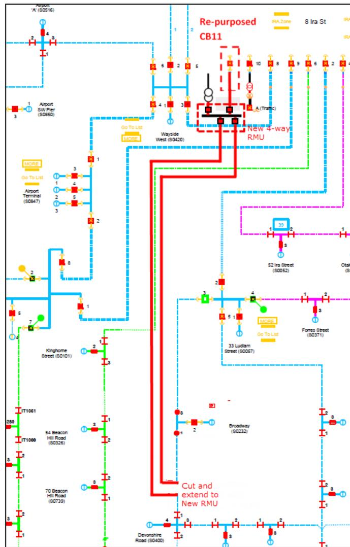
Figure 5-41 Ira Street Feeder 2 Reinforcement Project
