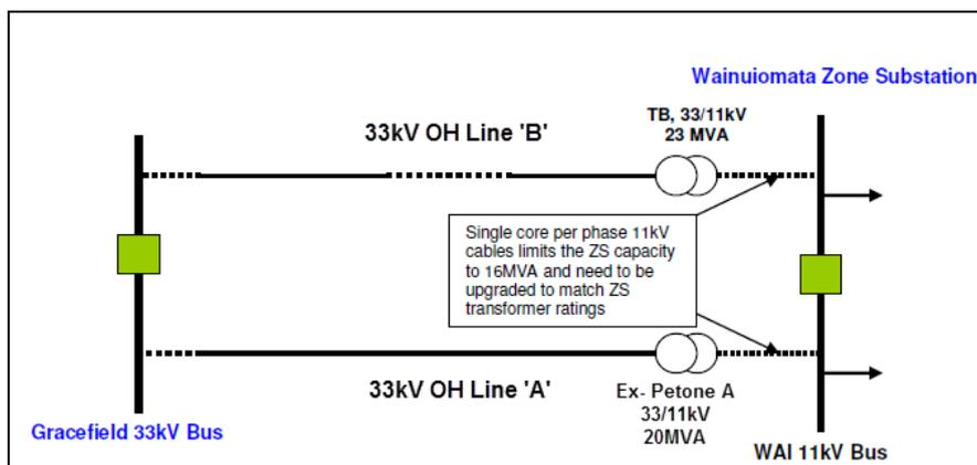
Figure 5-32 Wainuiomata Zone Substation Layout
