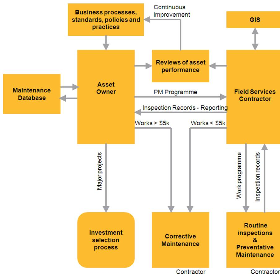
Figure 2-14 Inspection and Maintenance Process
