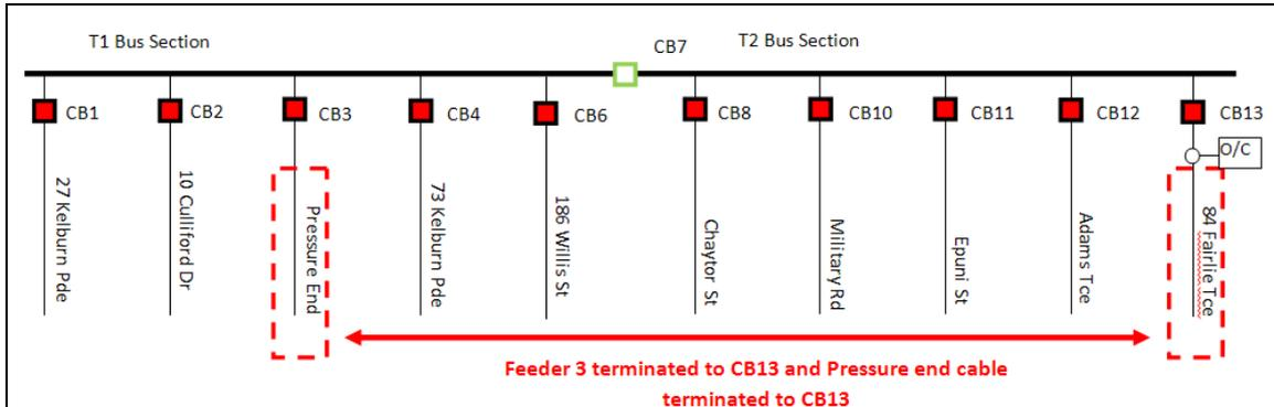
Figure 5-53 Re-configuration of the University zone substation
