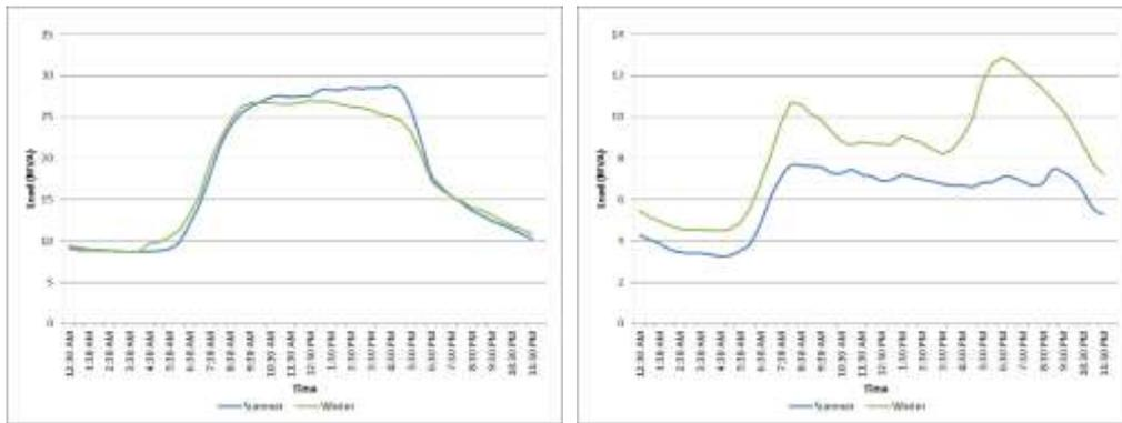
Figure 3-5 and 3-6 Typical CBD (L) and Residential (R) Zone Substation Daily Load Profile
