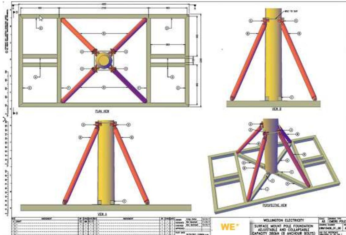
Figure 8-20 33kV Pole Structure Supports (Example only)
