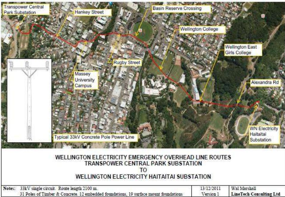
Figure 8-19 33kV Emergency Overhead Line Corridors (Example only)
