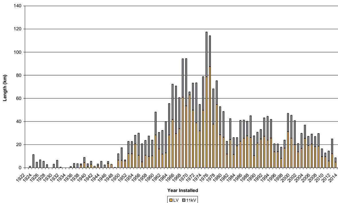
Figure 3-44 Age Profile of Distribution Cables
